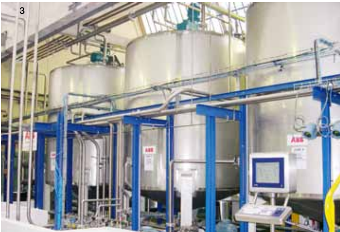
1 Powder conveying screws on metering hopper | 2 Piggable manifold with pig loading stations | 3 Storage tanks in Atex area with operator terminal | 4 Piggable collectors to precisely dose liquid materials through mass-flow meters
