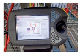
SafeMove opens up for man-machine collaboration. The operators and the robots can work together without compromising on safety. It uses geometrical and speed restrictions, maintaining automatic operation. This combines the flexibility of human interaction with the precision and handling capacity of robots. SafeMove brings great savings on floor space by restricting robot motion to precisely what is needed by the application.
