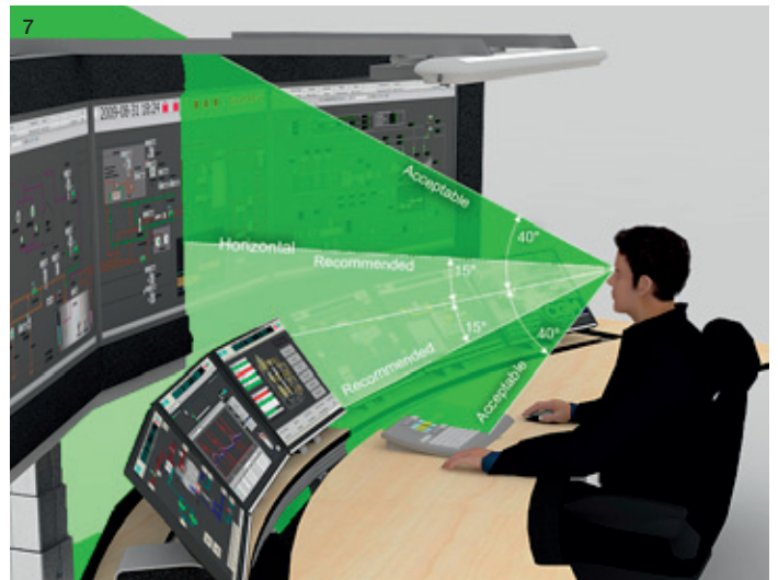
Fig 6. Adjusting EOW-x screen position and distance reduces stress on the eyes as well as viewing muscles. | Fig 7. Vertical field of vision for monitoring (sitting position). | Fig 8. Vertical field of vision for detection (sitting position). | Fig 9. Vertical field of vision for detection (standing position). The light green areas show the recommended field of vision, the dark green the acceptable field. EOW-x fully complies with the EN 894 standard.
