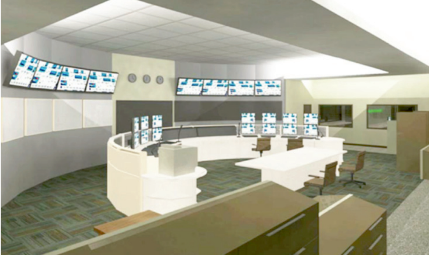
Fig 1. A traditionally-planned central control room with two-tier monitor stacking and larger screens mounted on a distant wall or stand. Arrangements like this put a strain on operators and may compromise their ability to work effectively.
