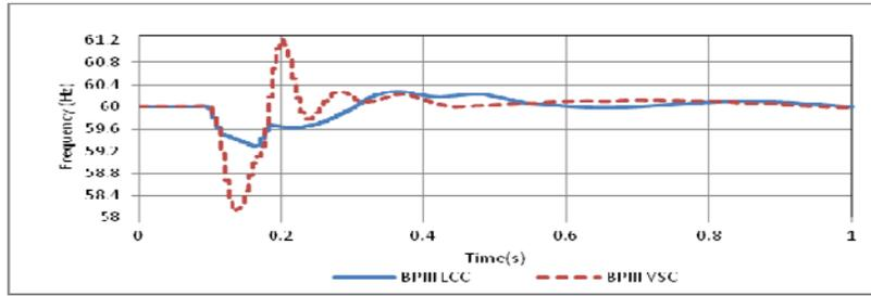
Figure 7: Frequency dip at Riel for a rectifier AC fault – 2000 MW Bipole III.
