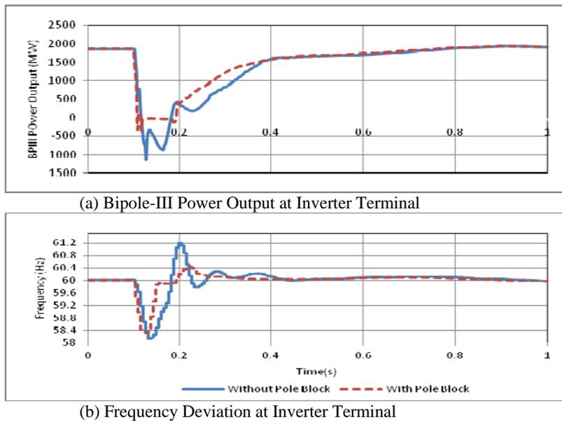
Figure 10: Frequency changes at inverter terminal due to reverse power of 2000 MW VSC option for Dorsey-out powerflow scenario.
