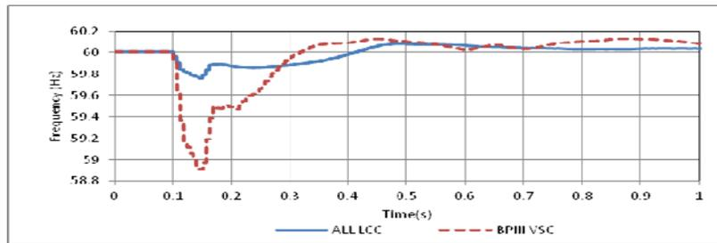
Figure 6: Manitoba southern system frequency response to a DC line fault.
