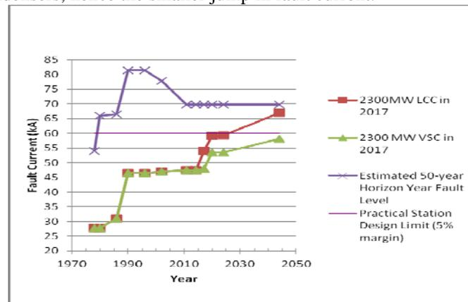
Figure 1: Fault current growth at Dorsey 230 kV substation, Winnipeg.
