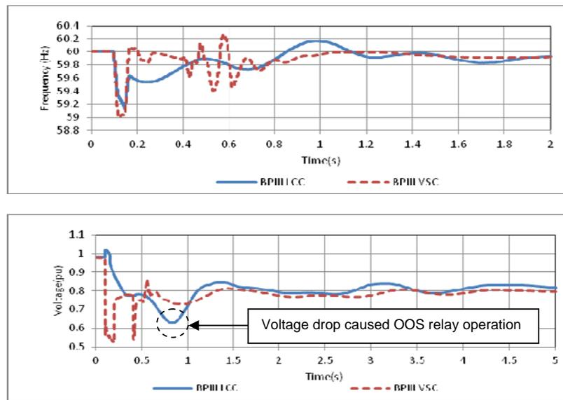
Figure 11. Bipole III block (2500 MW) with Dorsey out; Out-of-step relays blocked from line tripping. Top: Frequency response; Bottom: Glenboro 230 kV voltage.
