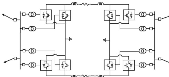
Figure 4: Bipole 3 conceptual single line diagram assuming voltage source converters.
