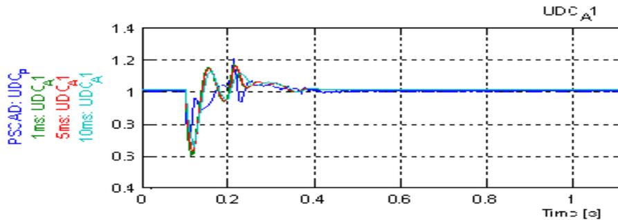
Figure 3: Sample graph from comparison between PSS/E model and full PSCAD model. 3-phase short circuit at rectifier with <10% remaining voltage.
