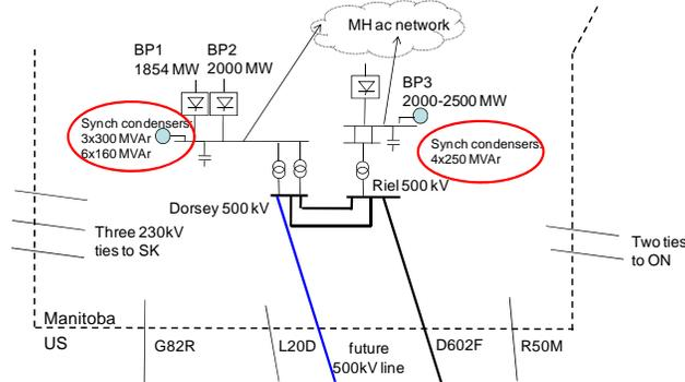
Figure 2: High level diagram of Manitoba Hydro's southern system DC inverters and tie lines.
