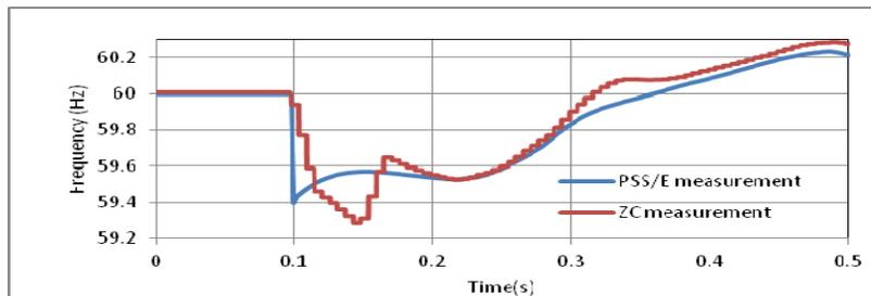
(b) Frequency Measurements (PSS/E uses 50 ms low pass filter)
