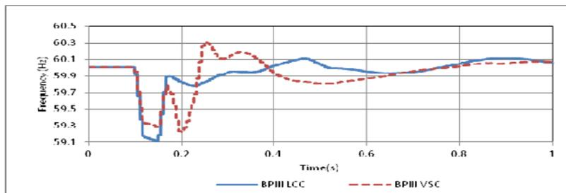
Figure 8: Frequency dip at Riel for an inverter AC fault – 2000 MW Bipole III.
