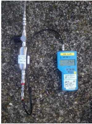
Figure 2. Gas sample cylinder with digital pressure indicator, DPI 705, connected before sampling.
