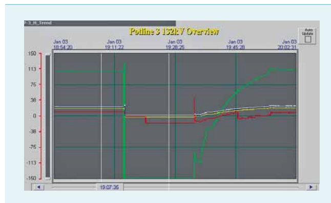
1 Active power demand during potline trip and start-up
