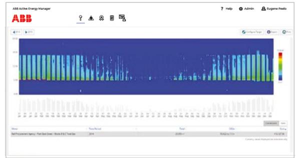
The profile of the graph demonstrates tight control of gas consumption outside of core office hours (dark blue colour) and low gas consumption in summer months (middle of the graph) as indicated in the previous graph.
