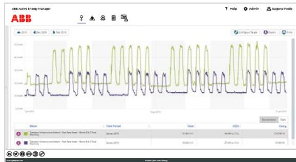
Savings as a result in a fall in baseload consumption as indicated by the purple line (2014) being lower outside of core operating hours than the green line (2010)
