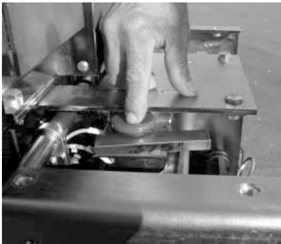
Figure 33. Trip coil button with gage
