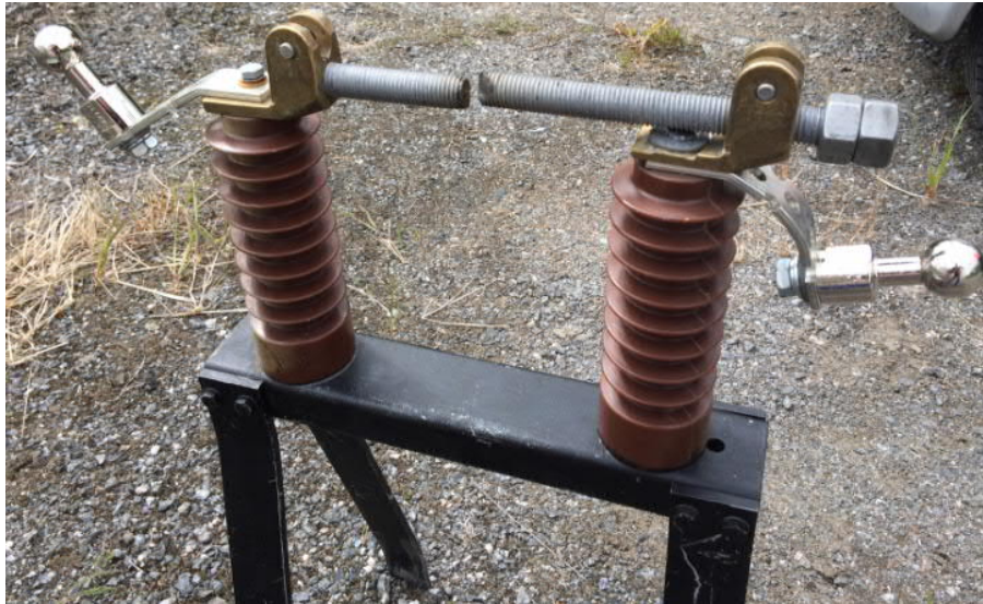
Figure 3. Test equipment for intermittent earth faults
