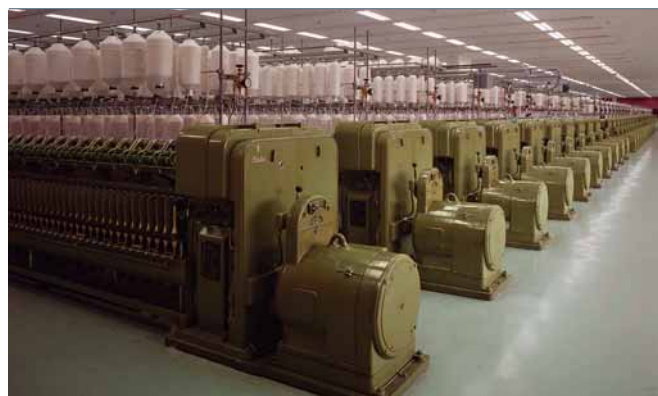
5 Three-phase shunt commutator motors with pipe ventilation and built-in spinning regulators (1965)
