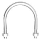
PC02 - Pipe clamp (1 pair) Pipe clamp (M8*60mm) for pole Ø2-3/8" (60mm)
