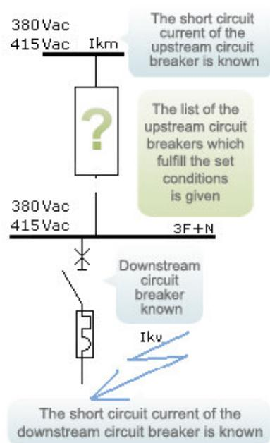
The user is guided through the identification of the circuit-breakers by filling in the different fields, which has to be made in sequence.
