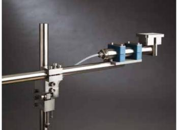
L&W Consistency Meter is a portable instrument from Lorentzen & Wettre, designed to analyse, make more efficient and optimize dewatering in paper, board and pulp machinery. L&W Consistency Meter is used to measure the amount of water at various stages after the forming section, to see if all the dewatering elements are correctly adjusted in relation to the product that is currently being produced.
