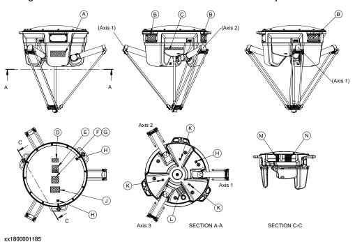
Α **ABB** logotype В Transport protection label 3 pcs С Label, FlexPicker D UL/UR label Ε Lifting instruction label F Rating label (2 pcs) G WEEE label Н Warning label - Electricity (symbol of flash) (3 pcs) Instruction label Before dismantling see product manual Κ Axis marking L Instruction plate, brake release М Calibration label Ν Rating label
