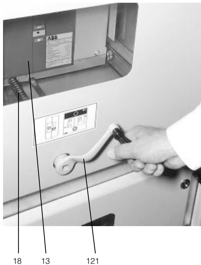
Figure 6/6: Movement of the withdrawable breaker part between the test/disconnected position and the service position, with approx. 20 turns of the crank, clockwise up to the stop for the service position and anti-clockwise for the test/disconnected position
