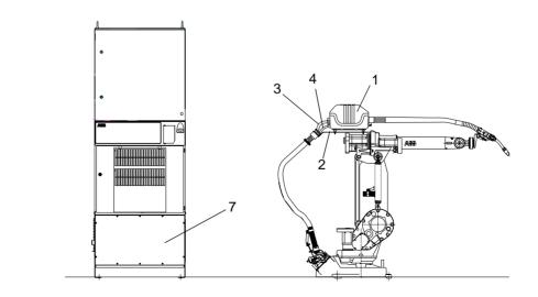
Figure 7 Robot Welding System with integrated power source.
