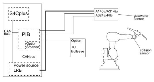
"ARCITEC" with integrated power source LRB400, or separate LRC430
