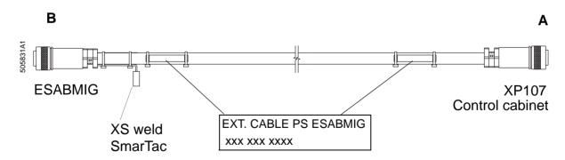
Figure 14 Control cable ESABMIG
