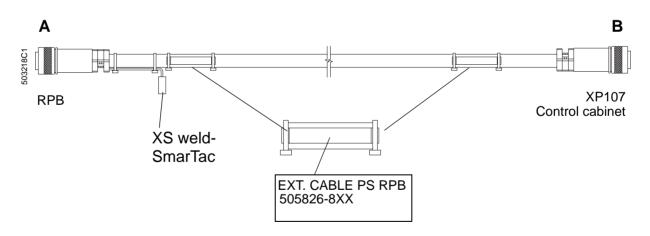
Figure 15 Control cable RPB.
