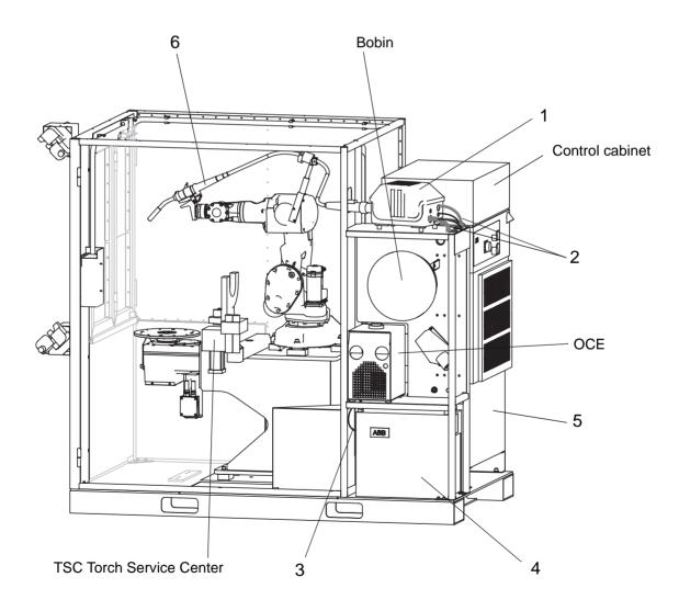
Figur 5 Robot Welding System with separate power source.
