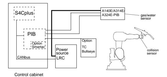
Figure 4 Overview of "ARCITEC" connections LRC.
