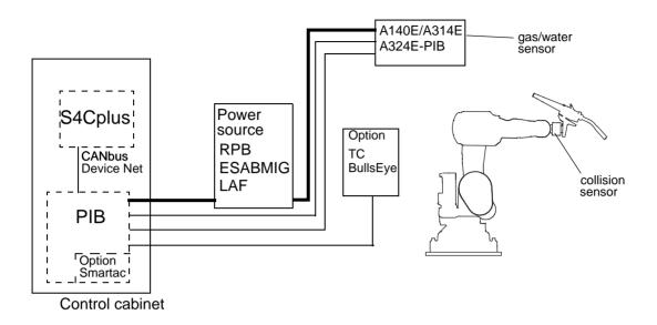
Figure 2 Overview of "Flexible Interface" connections.
