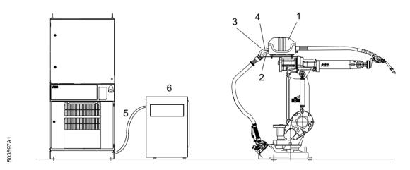
Figure 6 Robot Welding System with separate power source.
