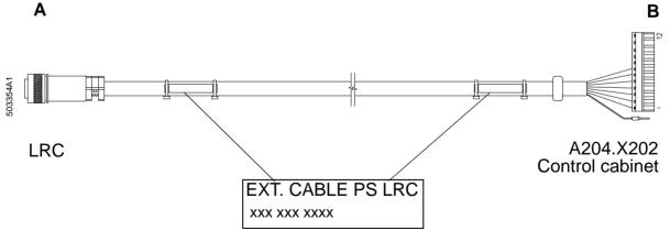
Figure 17 Control cable LRC
