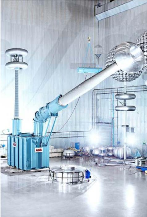
Figure 4. 1100 kV<sub>dc</sub> converter transformer prototype after passing all tests.
