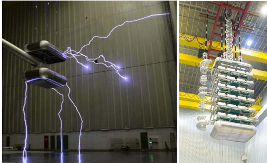
Figure 6. Breakdown test and type test of 1100 kV converter valves.
