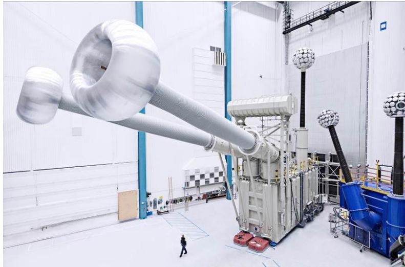
Figure 5. 1100 kV<sub>dc</sub> converter transformer for Changji station after type test.
