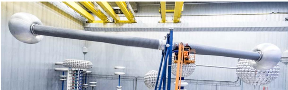
Figure 5. 1100 kV UHVDC wall bushings at test set-up.
