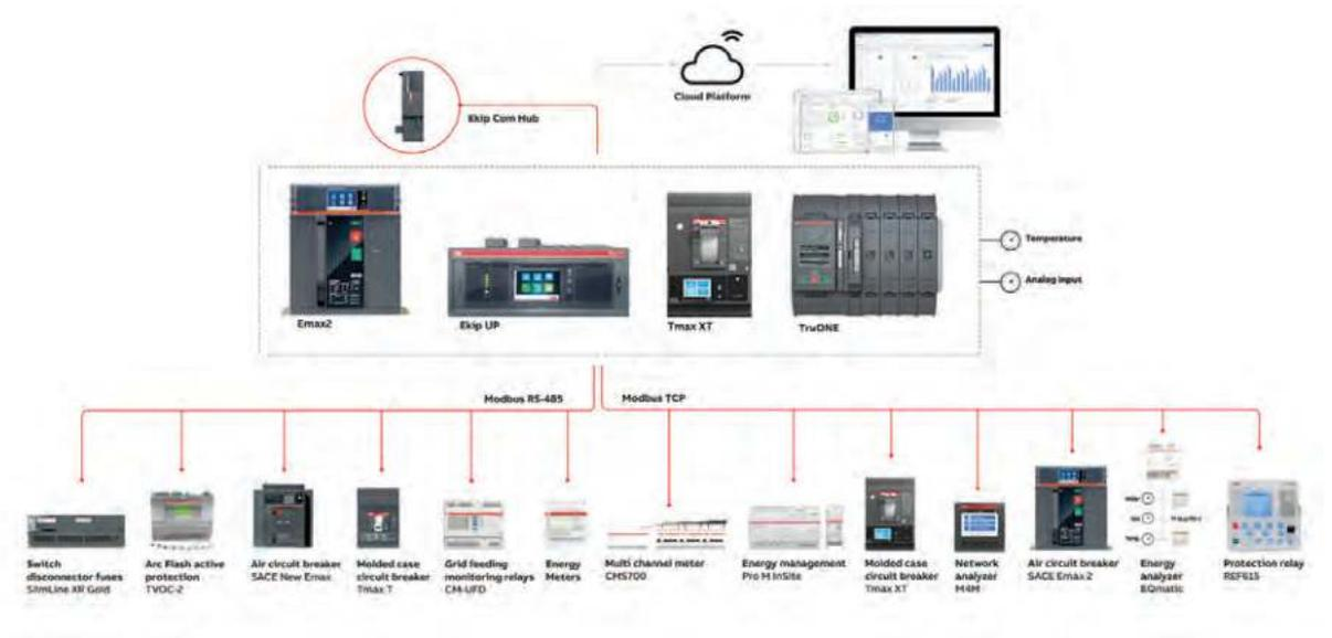
**External solution with ABB Ability™ Edge Industrial gateway**
