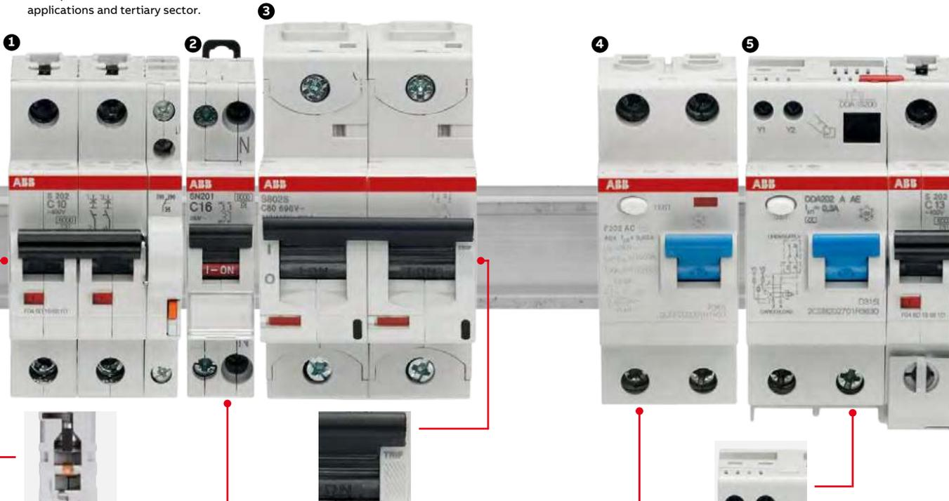
Increased terminal opening for higher wire gauges up to 35 mm<sup>2</sup>. For conductors with or without connector sleeves. Fulfills still the requirements for protection degree IP20 (finger safe) acc. to IEC/EN 60529. Integrated plate protecting flexible cables from damage and homogenous pressure in the terminal opening.
