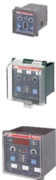
Front panel residual current relays are electronic devices used in combination with an external toroidal transformer. They are according to the protection standard IEC/EN 60947-2 Annex-M. The sensitivity can be set from 0.03 A to 30 A, while the tripping time from 0 to 5 seconds. Residual current relays are available in versions 48x48 mm, 72x72 mm, and 96x96 mm.
