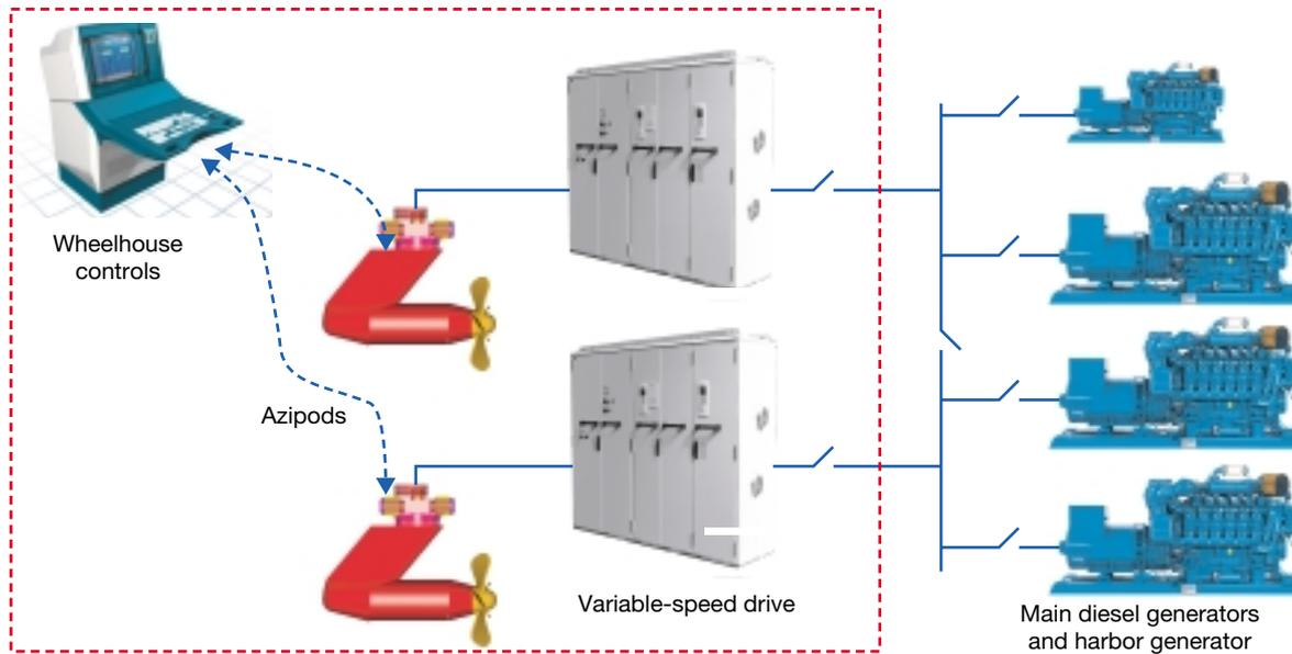
Azipod® (for Azimuthing Podded Drive) was developed to take advantage of all these characteristics and provide the kind of dynamic performance and maneuverability that today's marine market demands. The ultimate electric propulsion configuration, with Azipod units and variable-speed drives, is shown in **1**.
