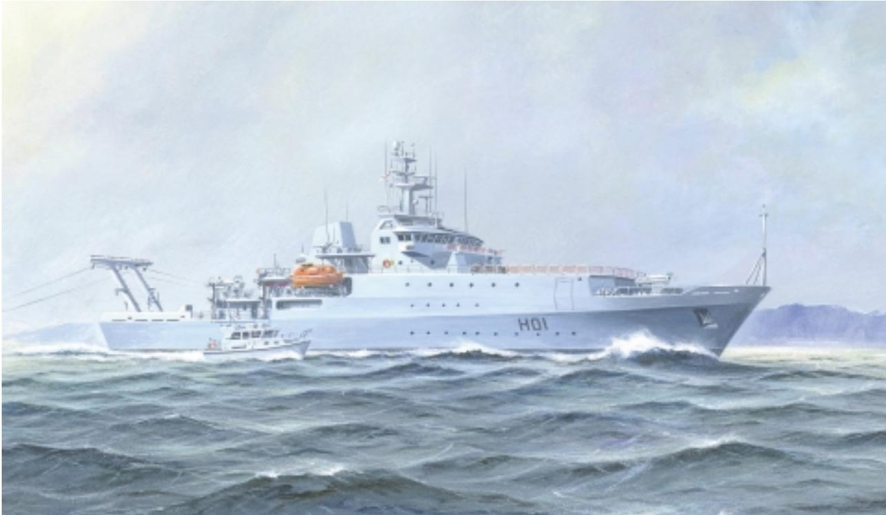
for the main power plant and two pulse width modulation DTC-controlled Compact Azipod units rated at 1,700 kW each. Key issues in winning this contract were the units' excellent propulsion performance and low life-cycle costs. The latter are the result of high diesel-electric propulsion efficiency and low-cost maintenance. The ships are the first Royal Navy vessels to have integrated electric and Azipod propulsion systems.
