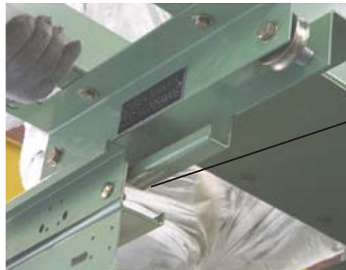
Figure 13. Align wheels on the front rail and behind the rear rail as shown.
