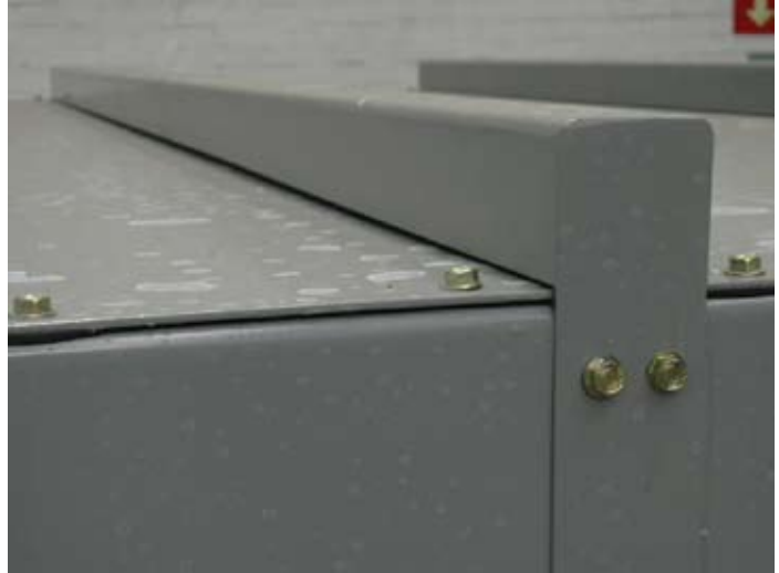
Figure 20. Tighten the shipping split angle evenly.
