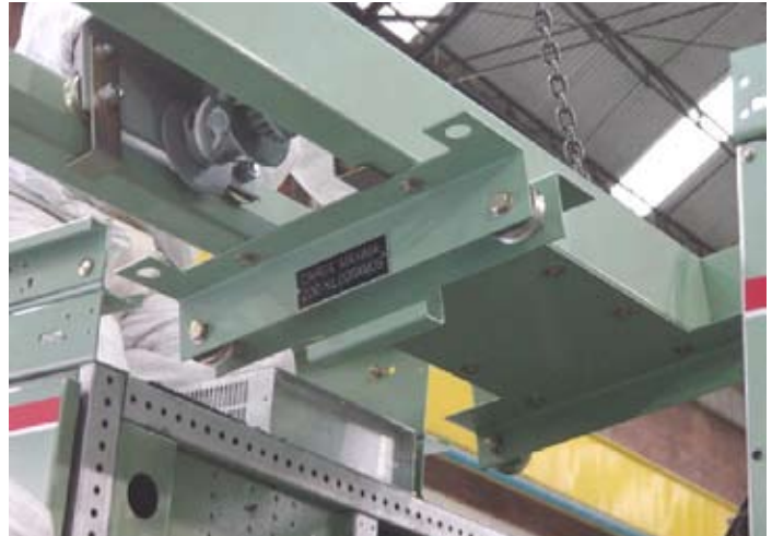
Figure 12. Lift the Overhead lift device up to the rails on the frame
