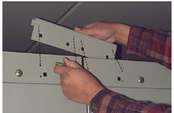
Figure 9. Mount Location Plate behind the rail.
