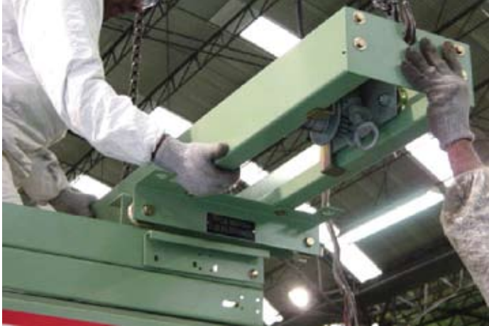
Figure 14. Push the Overhead Lift Device onto the rails.
