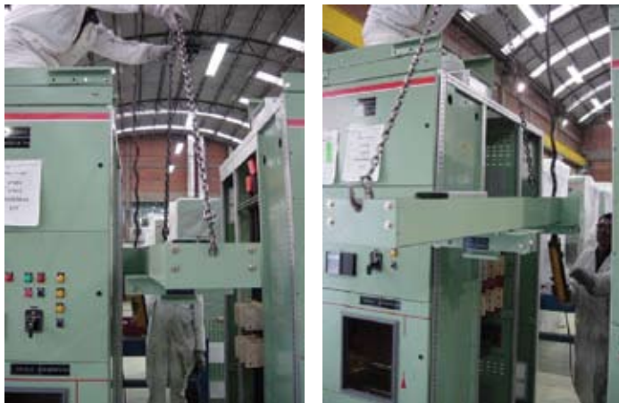
Figure 11. Position Overhead Lift Device on tines of fork lift.
