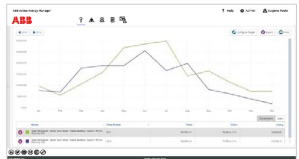
The time period comparison shows a drop in energy consumption of 17% from 2011 to 2012 which is due to more efficient operation of the AHU during store operating hours.
