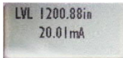
By pushing the UP or Down button, the main display can be scrolled to display the level in terms of a percentage of calibrated range (Figure 6) or in terms of a linearized / strapped measurement. (Figure 7).
