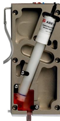
Figure 3 Electrode in temperature-controlled flow cell
