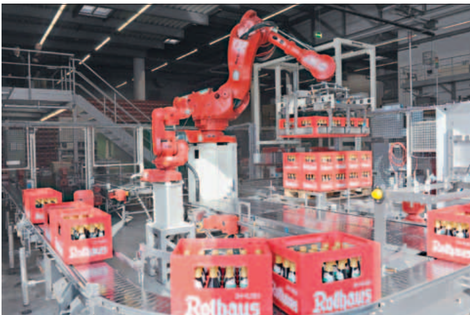
4 The smaller IRB 140 working alongside the larger IRB 6640 in the world-famous Rothaus brewery
