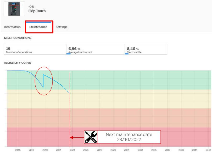
When maintenance is performed by an ABB authorized Field Service Engineer, the Predict function can also show the effects of maintenance performed
