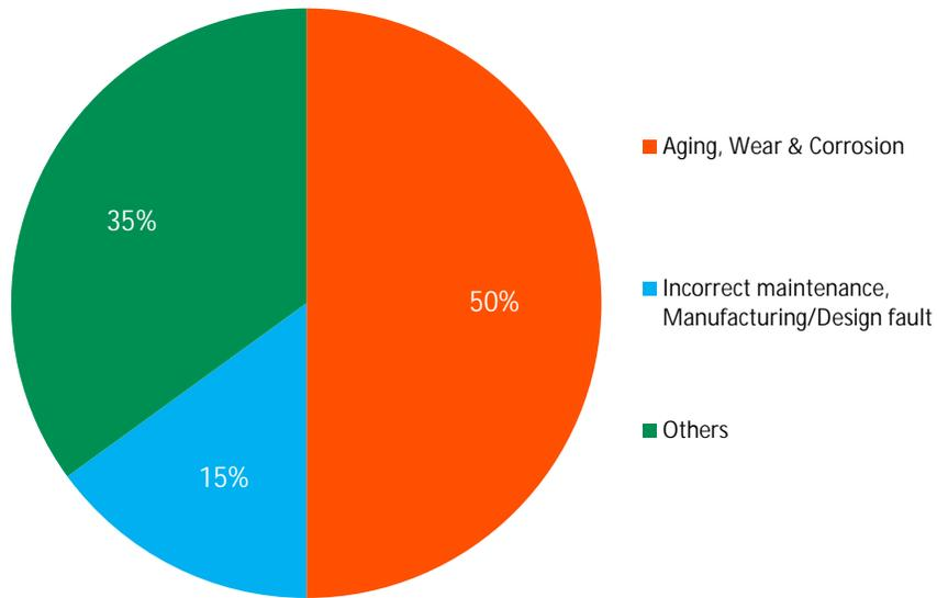
As per the International Surveys conducted by IEEE on Circuit-Breaker Reliability Data for Substation and System Studies, 50% of the time aging, wear and corrosion have been reported as common failure mode.
