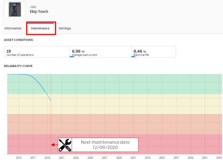
A Maintenance Page shows the circuit breaker's reliability curve according to the data collected and analyzed.
