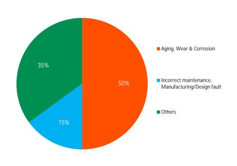
As per the International Surveys conducted by IEEE on Circuit-Breaker Reliability Data for Substation and System Studies, 50% of the time aging, wear and corrosion have been reported as common failure mode.
