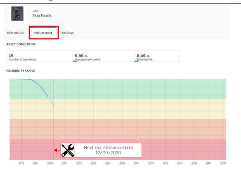
A Maintenance Page shows the circuit breaker's reliability curve according to the data collected and analyzed.
