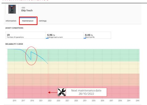
When maintenance is performed by an ABB authorized Field Service Engineer, the Predict function can also show the effects of maintenance performed
