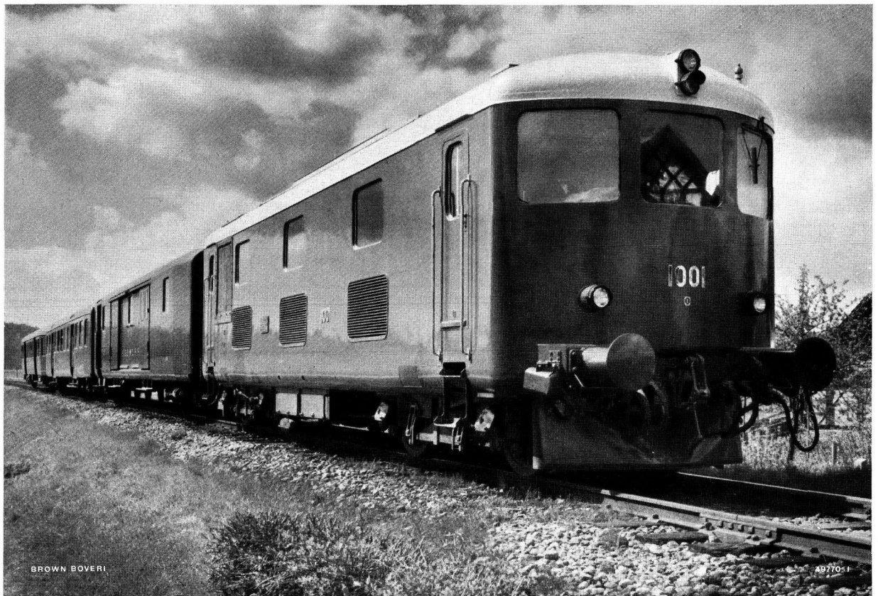
1200-H. P. Diesel-electric locomotive Bo-Bo, weight in service 65 t, Series Am 4/4 No. 1001 of the Swiss Federal Railways. Trial run with light trailer coaches on the Winterthur-Schaffhausen line section.
