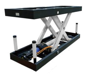
The FlexLifter IRL 600 is designed to improve accessibility of the part by adding a programmable degree of freedom to the Flextrack IRT501-66 track motion. It is possible to use the unit to position a part tooling in front of the process robots. The unit can also be used also as a standalone module.
