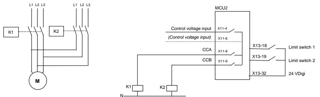
**Picture 27.** Control circuit for Actuator starter with torque switch, MCU2.
