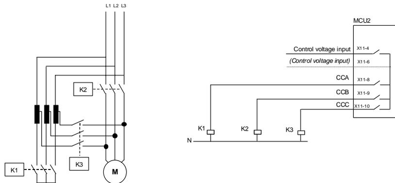
**Picture 30.** Control circuit for autotransformer starter, example 3.
