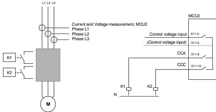
**Picture 16.** Control circuit with softstarter for REV-DOL, latched contactors.
