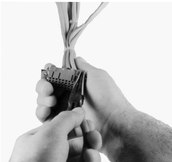
Fig. 1c. Adapter Bracket Locking Tabs
