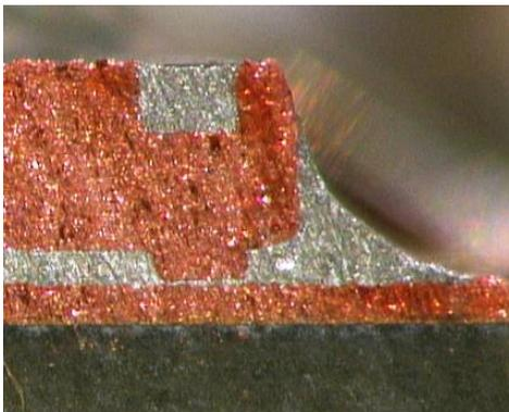
Fig. 1. Partial cross section of a terminal solder joint showing the new implemented spacers resulting in homogenous solder thickness.
