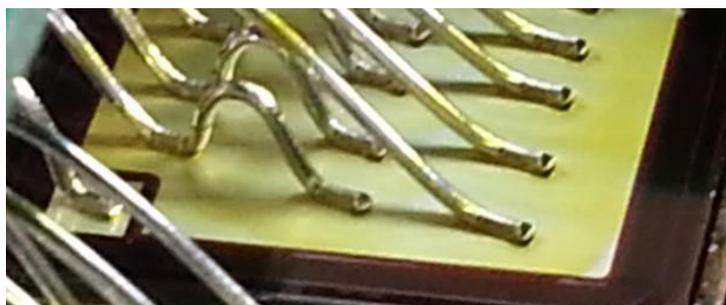
Fig. 3: New redundant bonded connection between substrate and gate-print
