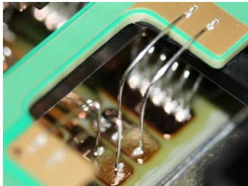
Fig. 2: New redundant bonded connection between substrate and gate-print
