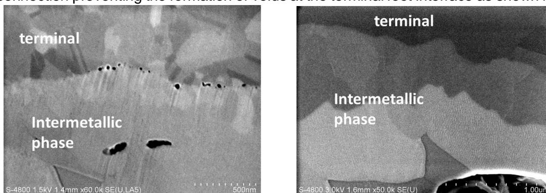
Fig. 4a.) SEM images of the former terminal solder joint showing void formation between the terminal-solder interface in the nanometer scale
