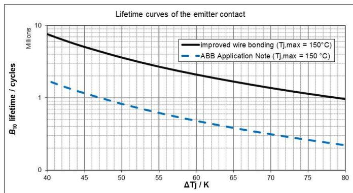
Fig. 5: The 10% power cycling capability curves ( $T_{j,max}=150^{\circ}C$ ) of the improved emitter contact and the previous emitter contact (given in the ABB application note [2])
