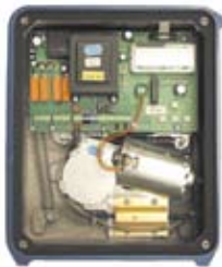
Electronic Chamber: Control system and processing of the measurement.
