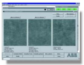
Changes in formation caused by such factors as jet to wire ratio variation, refining and other process parameters can be immediately viewed with the ULMA NTis web imaging snapshots
