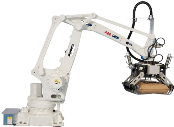
The FlexGripper-Claw is a simple plug-and-play extension to the ABB IRB 460 or IRB 660 palletizing robots for high-speed bag palletizing applications. Stainless steel parts make it perfect for use even in the harshest conditions.
