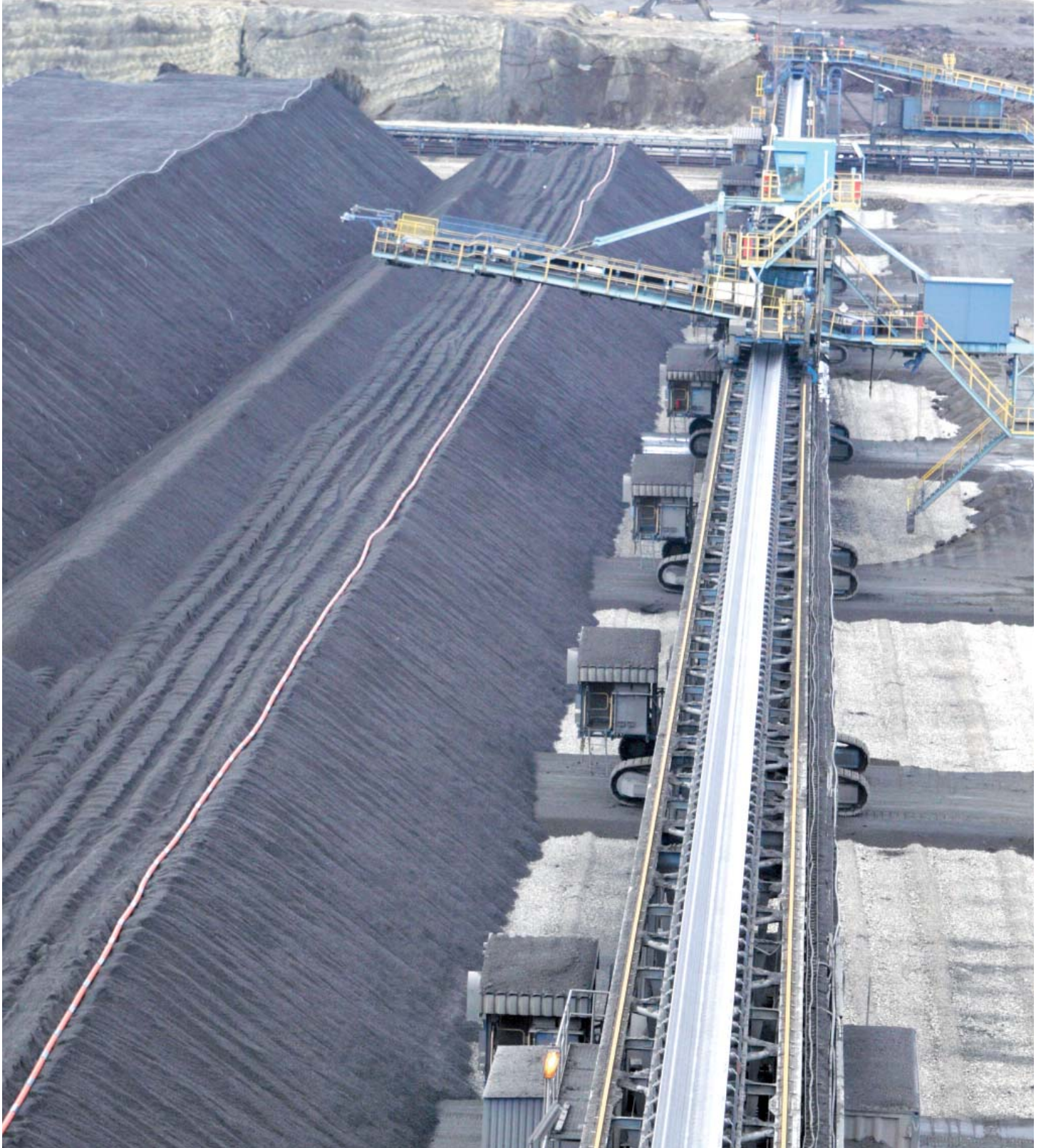
ABB drives help secure efficient stacking and reclaiming, ensuring the required quality of the blended material.
