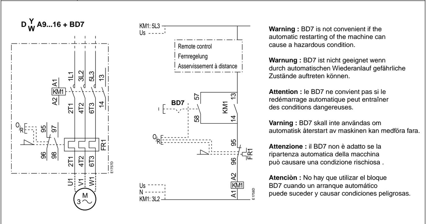
**Warning !** The operation, installation and servicing of this appliance must be carried out by a qualified electrician applying the relevant rules of the art, installation standards and safety regulations. Before operating the contactors, check that control voltage complies with the data on the coil mounting bracket. Connection to other control voltage can destroy the coil. Do not touch live parts. Danger !
