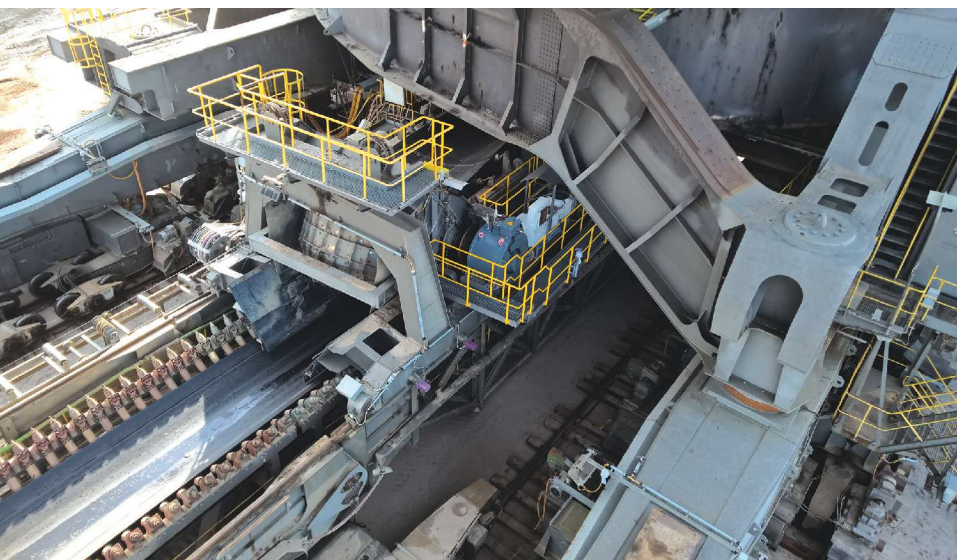
Setting precedents: ABB's gearless conveyor drive, center, offers up to 500 kN-m torque. (Photo: ABB)
