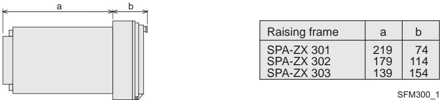
Fig. 3 Semi-flush mounting relay case (dimensions in mm)
