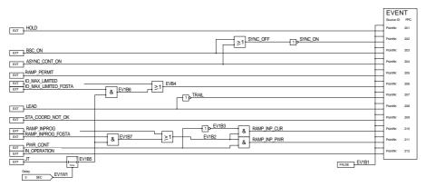
A typical event interface is shown. DPI symbols for set point adjustments and mode shift ordering are also shown below.
