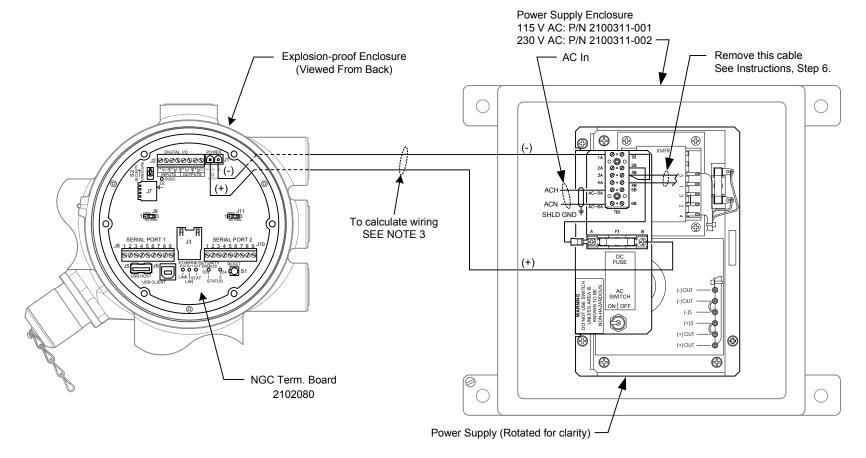
3. Wire size is a function of the distance between the NGC and the DC Power Supply. With the condition of a single heater used by the NGC, use 4 Amps as the maximum current draw to calculate an adequate wire size so that the voltage measured at the NGC's Power I/O terminal is a minimum of 12.5 Volts.
