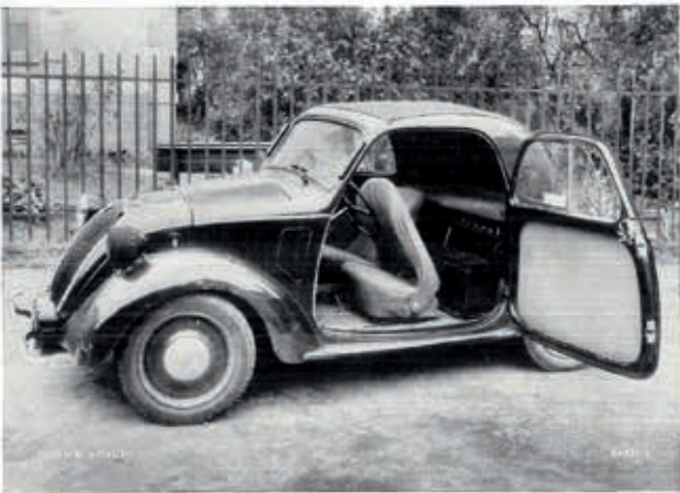
Fig. 146. — Passenger motor car converted to electric drive "Fiat 500 Topolino". Output 4.2 H.P., lead battery 90 Ah (for ten-hour discharge), 54 V, showing how the battery is built in. For short trips in towns with moderate inclines. Maximum speed attained on the flat 60 km/h.
