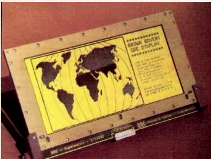
Prototype of a patented passive-matrix super-twisted nematic LCD with 540 × 270 pixels
