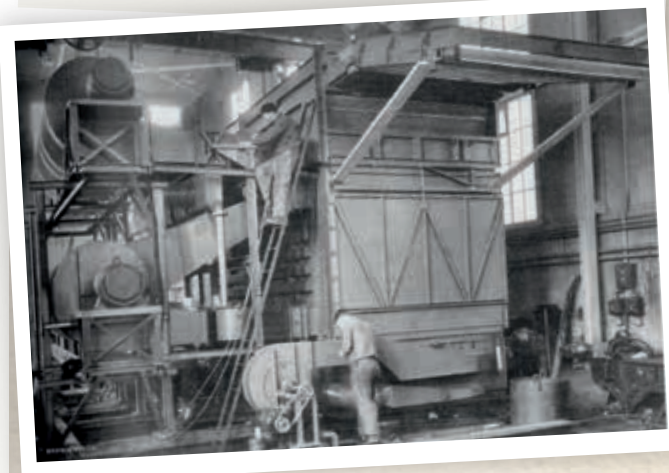
Fig. 6. — Electric grass-drying apparatus with heat recuperation. For an evaporation of 1000 kg of steam the power input is 400 kW. (A drying apparatus of same output, without heat recuperation would take at least 1200 kW.) 1. Charging belt (can be replaced by grab-hoist) for charging. 2. Drying sheets with built-in coverings and doors for cleaning. 3. Fan set with electric air heater and heat exchanger. 4. Discharge belt. Three machines of this kind ordered from us for delivery by the summer of 1941 will provide concentrated fodder for about 2000 head of cattle. The artificial drying of grass with heat recuperation is not only important to-day but is a process which is destined to play an important part in our food-supply problem of the future.
