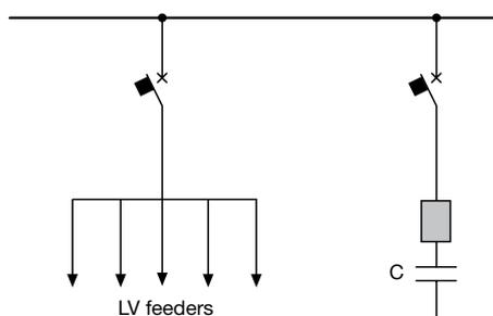
In centralized power factor correction automatic assemblies are normally used (see below automatic power factor correction) with banks divided into steps, installed directly in the main distribution boards; the use of a per-
