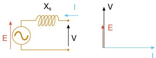
E : e.m.f. induced in the stator phases
