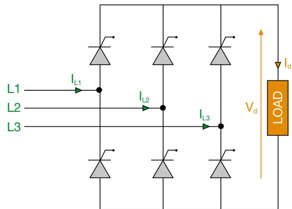
The current in each phase of the line (assuming a high inductance value on the d.c. side) has a rectangular waveform with the fundamental harmonic frequency equal to that of the sinusoidal voltage. The development in Fourier series of such waveform gives only harmonics<sup>6</sup> of order  $k = 6n \pm 1$  ( $n = 0, 1, 2, \dots$ ), whose theoretical amplitude is inversely proportional to the harmonic of order  $k^7$ , that is:
