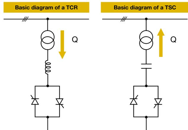
TSC allow a step-by-step control of the reactive power delivered by groups of capacitors, whereas with TCR a continuous control of the reactive power drawn by the inductors is possible.
