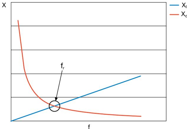
As shown in the graph, it is possible to observe that below the resonance frequency<sup>4</sup>  $f_r = \frac{1}{2 \cdot \pi \cdot \sqrt{L \cdot C}}$  the capacitive reactance prevails and consequently also the generated reactive power prevails over the drawn one, that is:
