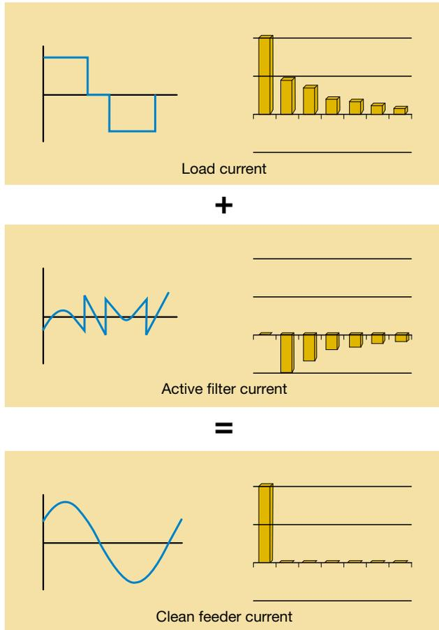
The active filter has the advantage of filtering simultaneously dozens of harmonics and does not involve design costs for dimensioning.
