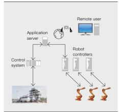
ABB's roboticsbased remote automation system prototype is capable of performing inspection and maintenance of an oil and gas process module.
