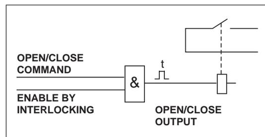
Fig. 8. Operation principle of OPEN and CLOSE outputs.
