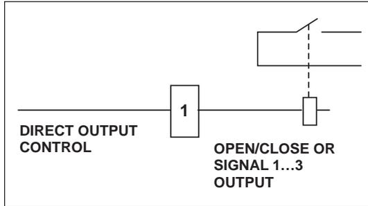
Fig. 11. Operation principle of Conditional Direct Output Control.
