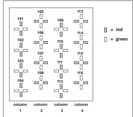
Fig. 6. Position, number and colour of the indicators on the front panel of SPTO 1D2.
