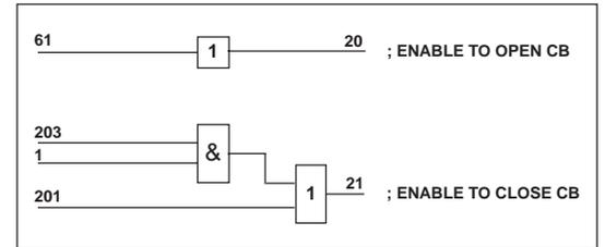
Fig. 19. Logic diagram for the default interlocking 10.
