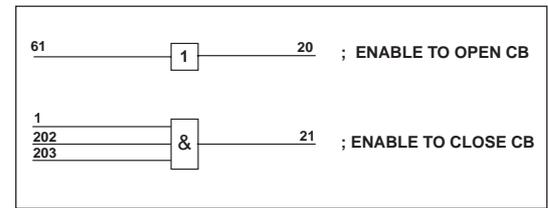
Fig. 17. Logic diagram for the default interlocking 2.
