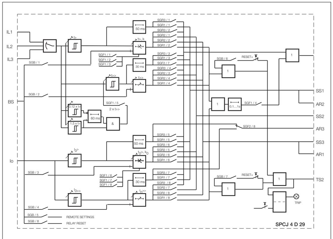
Fig. 1. Block diagram for the combined overcurrent and earth-fault relay module SPCJ 4D29.
