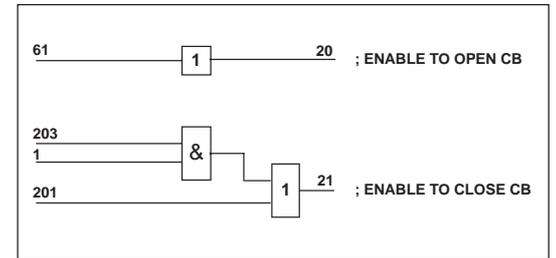
Fig. 15. Logic diagram for the default interlocking 1.
