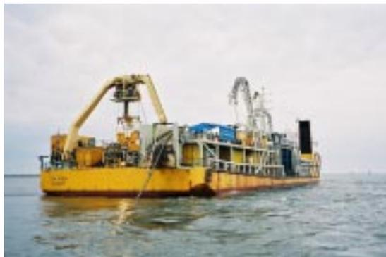
The cable was precisely laid on the seabed in the first crossing of the Sea Spider, a ship specially designed for submarine cable installation.
