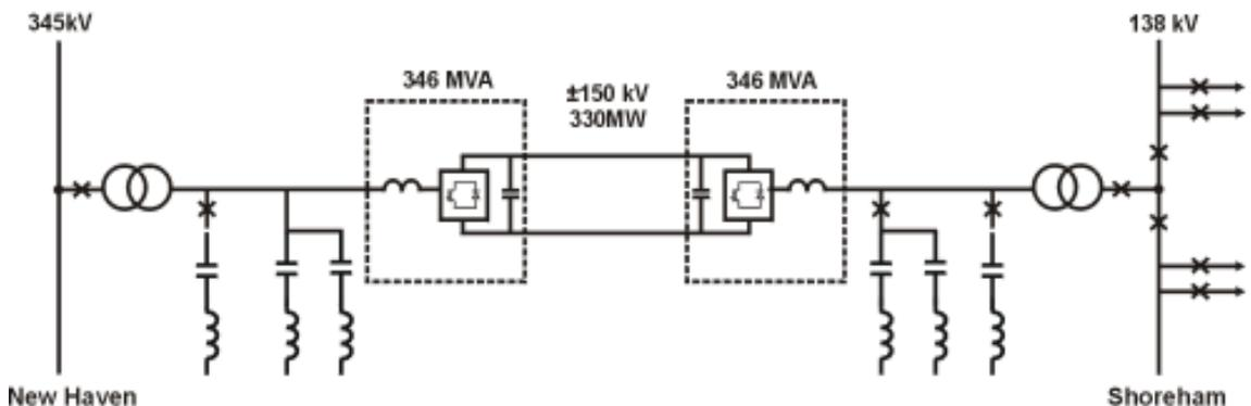
The Cross Sound HVDC Light transmission schematic
