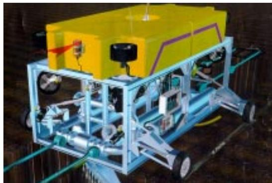
The Smartjet plow fluidized the seabed with pressurized water placing the cable six feet under the seabed.
