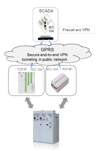
Figure 3. Communication Structure of the Smart Secondary substations
