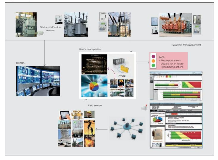
An expert system algorithm is then able to look at a transformer as a whole instead of at its individual components, as a health index would. technology (IT) software knowledge to provide the latest online offering in fleet condition monitoring.
