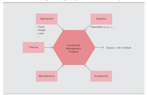
The algorithms employed by the DTMProgram are able to analyze each of the functional aspects of a transformer then aggregate these into the five functional areas used by the MTMProgram.
