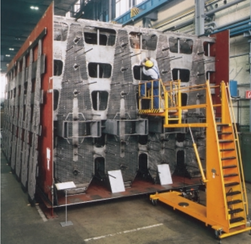
Turbine condenser module for the Lippendorf lignite-fired power plant being fabricated at ABB Kraftwerke GmbH, Berlin
