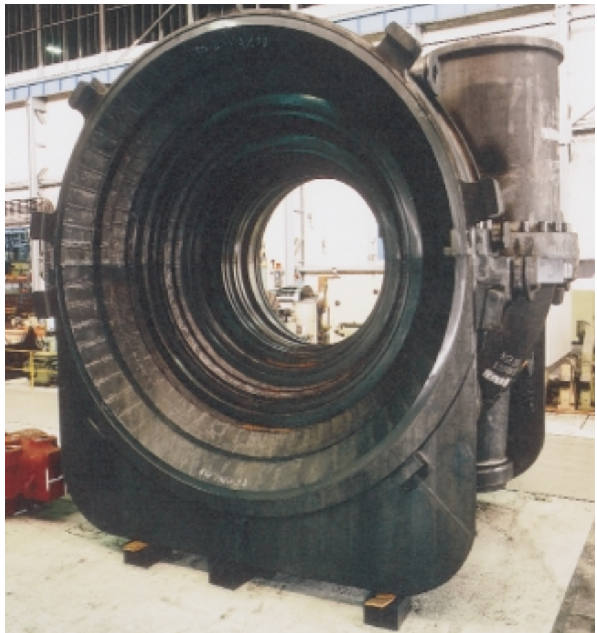
Nodular cast iron parts of the LP turbine inner casing after machining of the flanges
