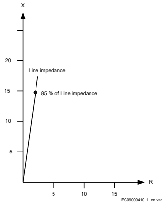
Figure 12: Line impedance diagram
