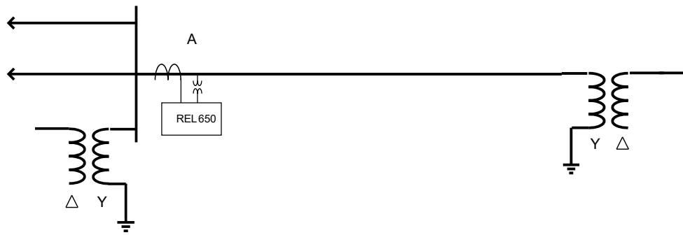
Figure 8: Two-ended over-head line with transformer in a solidly grounded network
