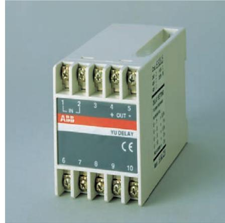
This allows circuit-breaker opening to be delayed (from 0.5 s to 3 s) when the power supply voltage drops or is cut off. It consists of a device (to be installed outside the circuit-breaker by the customer), which is interposed on the undervoltage release's power supply. The undervoltage release must be the type for direct current power supply.
