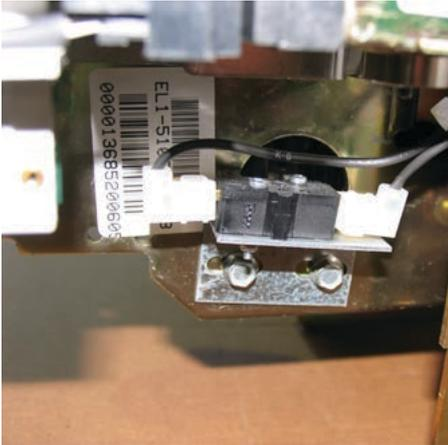
Two pairs of contacts (one open and the other closed) allow the status of the circuit-breaker's closing spring to be signalled in the remote mode. Only one contact can be wired, thus spring loaded or spring discharged can be signalled in the remote mode.
