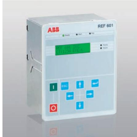
This protection device is an alternative to the similar PR521. Unlike PR521, which is self-supplied, REF 601 needs auxiliary voltage in order to function. On request, it can be equipped with all the HD4 series circuit-breakers with lateral operating mechanisms. It is the only protection device that can be installed on the HD4/R-Sec and HD4/L-Sec versions.
