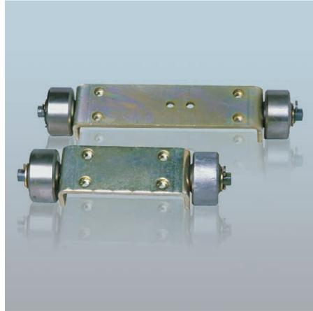
This kit consists of the front and rear wheel unit which can be assembled instead of the fixing brackets of the HD4/R and HD4/RE version of the circuit-breaker.
