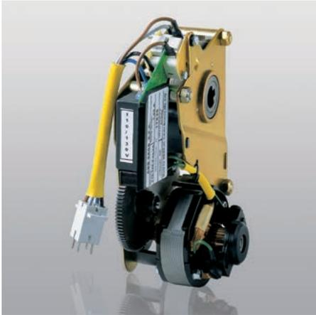
Automatically loads the closing spring of the circuit-breaker's operating mechanism. The gearmotor immediately reloads the closing spring after the circuit-breaker has closed. The closing spring can still be loaded in the manual mode (using the relative lever built into the operating mechanism) in a power failure or during maintenance work.
