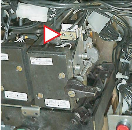
Installed in an electric circuit, this indicates the state of the undervoltage release.
