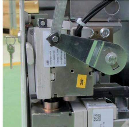
The shunt closing release (-MBC) allows the device to be closed by remote control. The release can function with both direct and alternate current and is fit for both instantaneous and continuous service. When permanently energized, the release provides the electric anti-pumping function. In the case of instantaneous service, the current impulse must last at least 100 ms.
